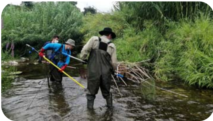
Sampling fish by electrofishing in the Serpis River near the city of Gandia (Valencia).
